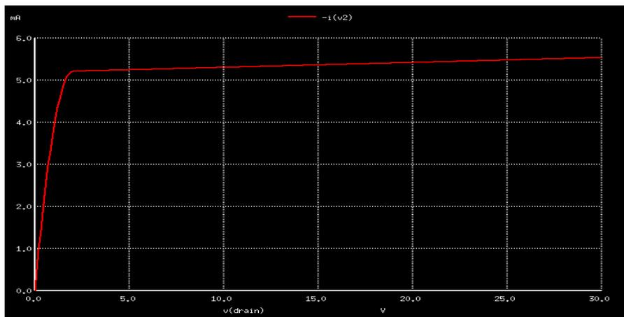
Figure 8.11: The drain characteristics of JFET with gate voltage =1V
