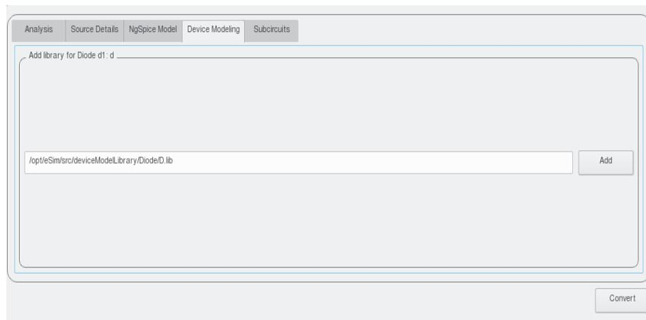
Figure 2.15: Choose the required diode model
