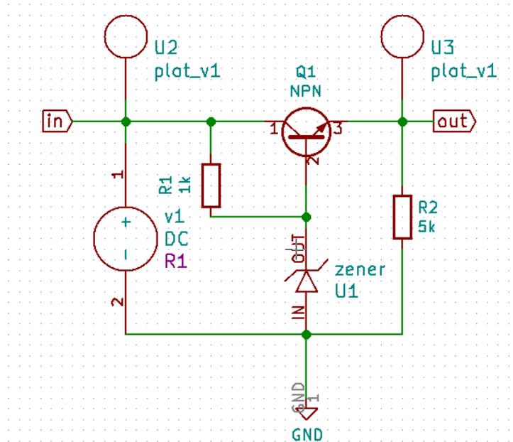
Figure 12.10: Schematic diagram for Zener Diode Regulator
