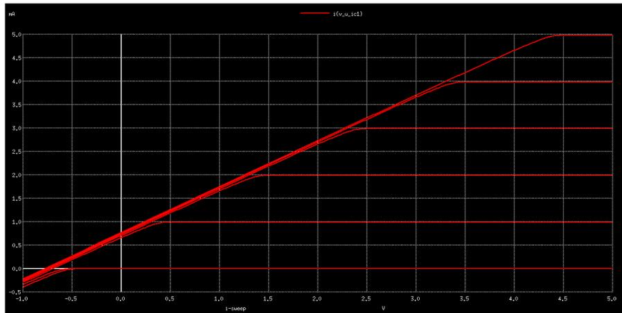
Figure 11.8: The output characteristics of NPN transistor
