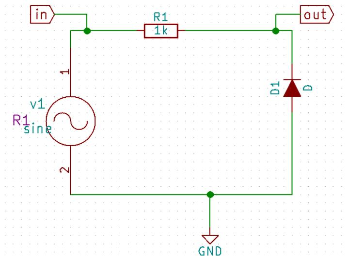
Figure 4.2: Schematic diagram for shunt clipper circuit
