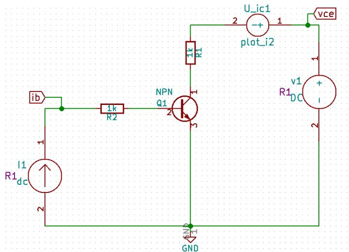
Figure 10.1: Schematic diagram for CE output characteristics
