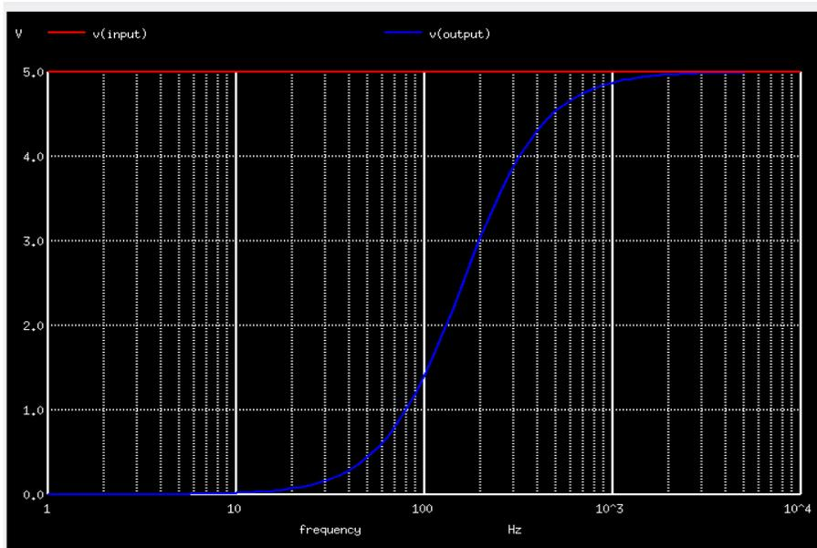
Figure 3.9: The frequency response of RC highpass filter
