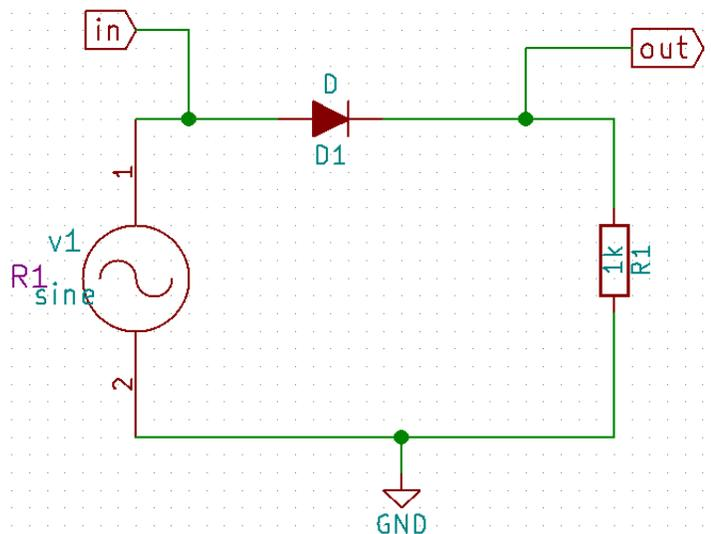
Figure 4.1: Schematic diagram for series clipper circuit
