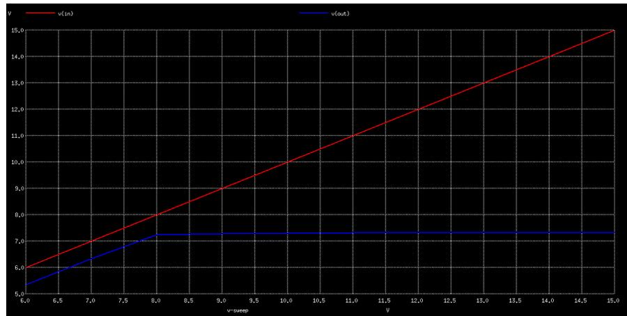
Figure 12.17: The line regulation characteristics of zener diode
