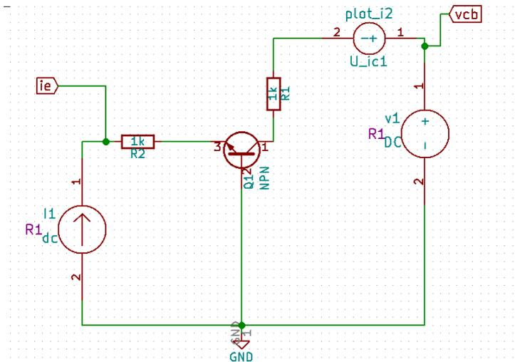
Figure 11.1: Schematic diagram for CE output characteristics
